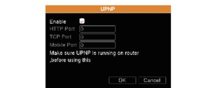
The DVR will auto configure the port forwarding of media, HTTP ports on the router. Make sure the router also enables UPNP function.
