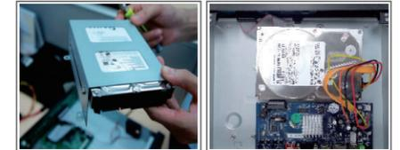
**03** Connect the SATA data and power cable to the HDD and the mainboard
