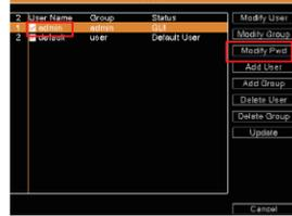
Leave blank for the old password, enter the new password and click "OK" to complete the modification.
