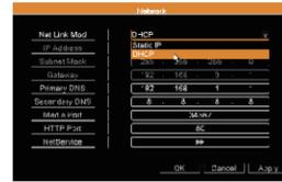
Set the correct IP address, subnet mask and gateway. Keep the default settings for other network parameters unless modification is necessary. And then click **Retry** to test network again until network test OK.
