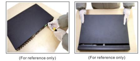
**02** Install and fix the HDD with the screws into the bottom panel of the DVR
