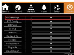
The DVR will detect the new HDD and you will see the R&W Disk from the list. Select the R&W Disk > click on Format Disk > select "OK" to delete all data. The interface will be frozen for a few seconds, please wait a few second to finish formatting.
