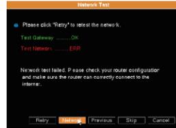
**04** Click Network to setup network parameters when network test failed.
